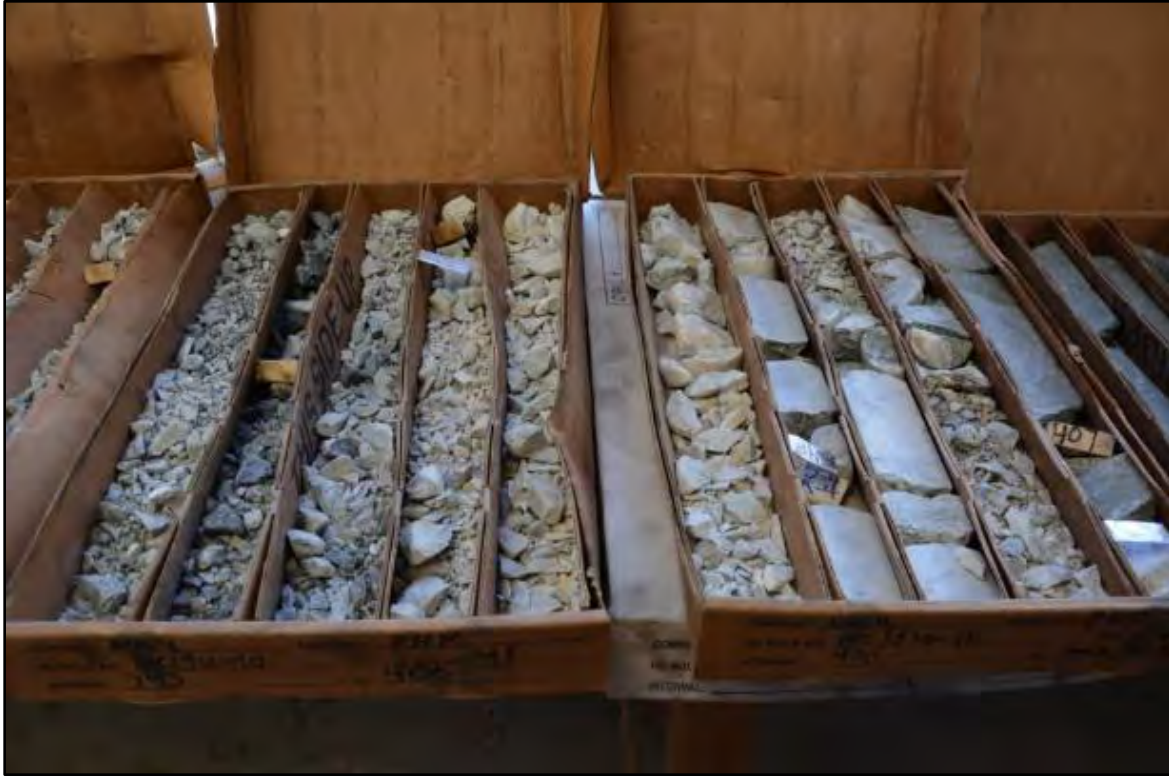
Figure 16-1: Example of Variability of Marble over Short Distance (Drill hole NC15-10, 393-442 ft)
